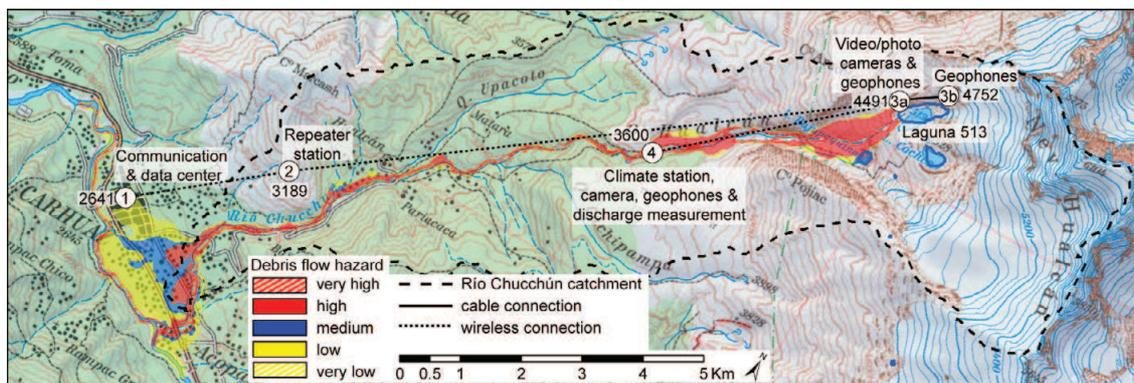
Figure 1. Río Chucchún catchment above the city of Carhuaz with the updated hazard map and the stations of the monitoring and early warning system (background: Alpenvereinskarte 1:100,000).
