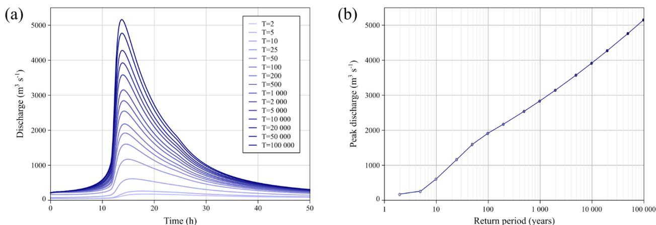
5 **Figure 9: (a) Resulting flood hydrographs for return periods between 2 and 100 000 years, for the Base Case. (b) Flood frequency characterization of the maximum values of peak discharges.**
