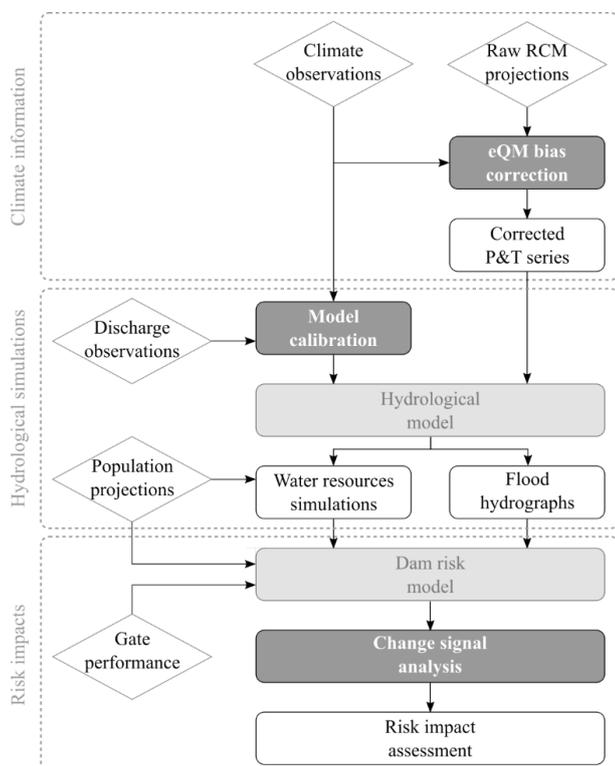
**Figure 1: Workflow of the methodology followed to assess the climate change impacts on dam failure risk.**
