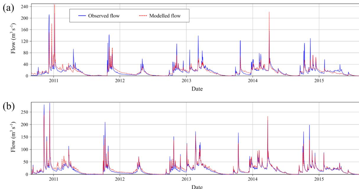
**Figure 6: Comparison between observed (blue) and modelled (red) flows for the gauging stations (a) Barco de Ávila, and (b) Puente Congosto.**
