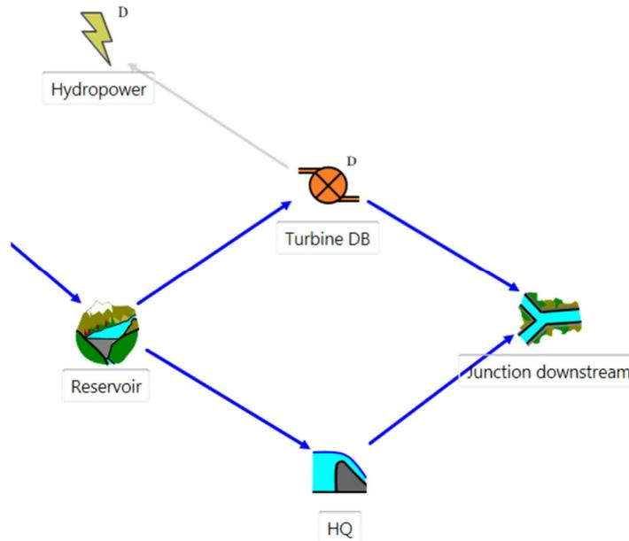
**Figure 22** Addition of a spillway
