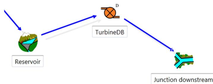
**Figure 17** Addition of a *TurbineDB* and a junction
