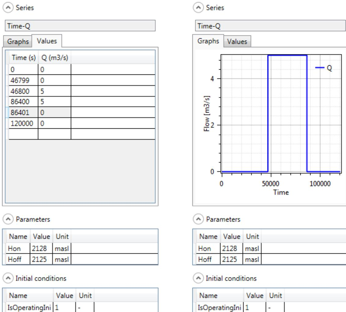
**Figure 114** Proposed release from the Turbine 2
