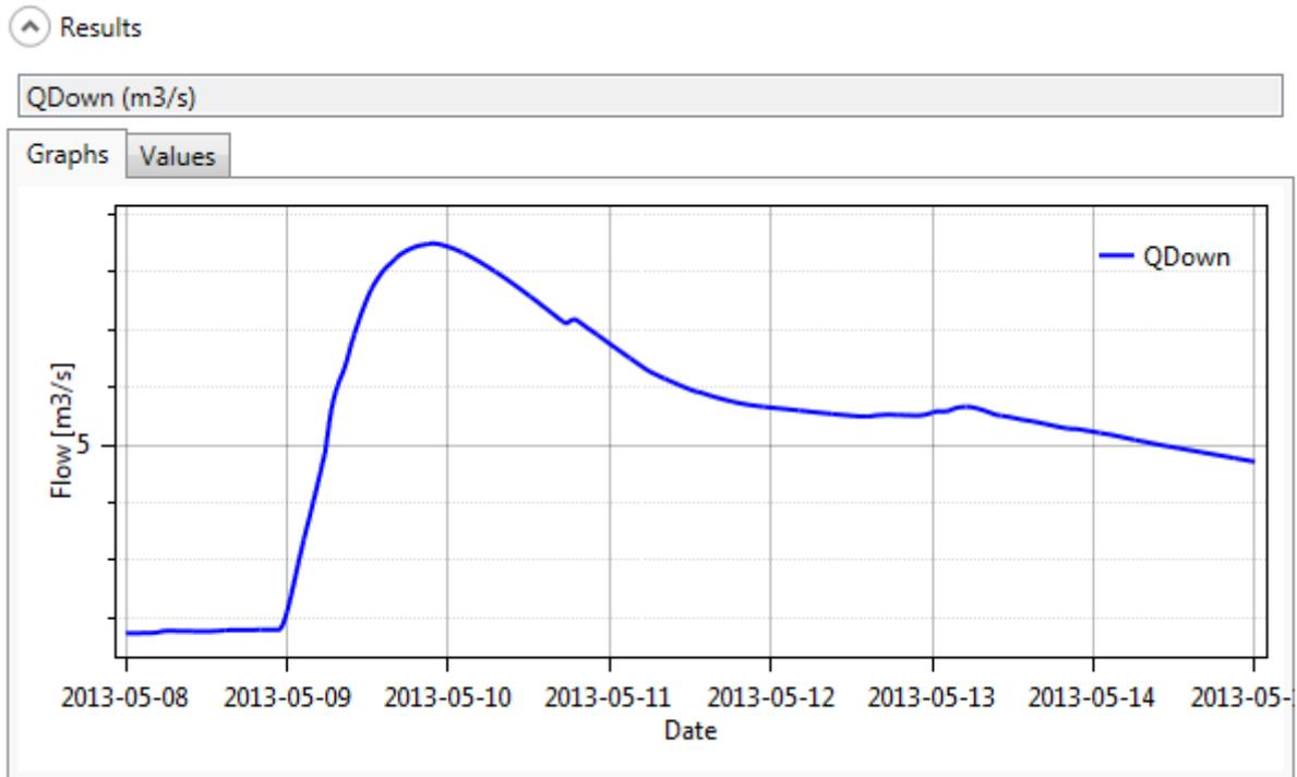
**Figure 111** Outlet hydrograph
