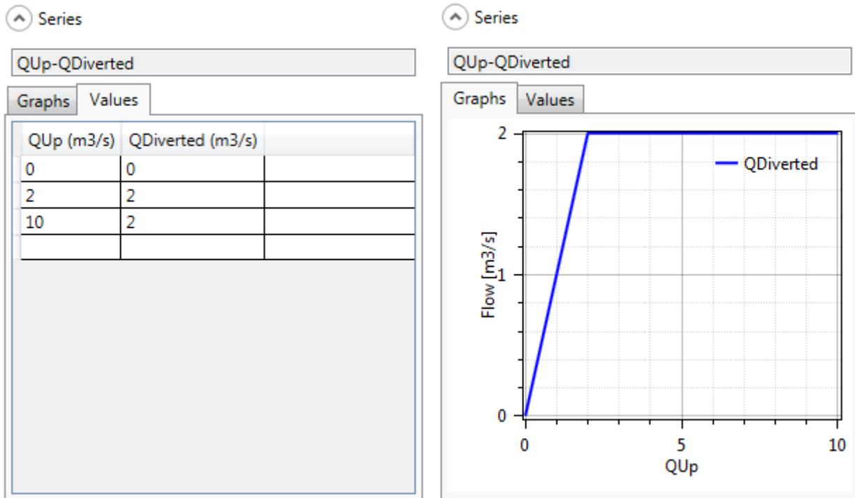
Figure 106 Relation Qup-Qdiverted introduced in the Diversion 1
