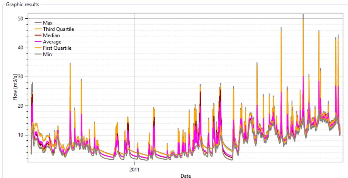
**Figure 67** Graphic results of the stochastic simulation, statistical series plots.
