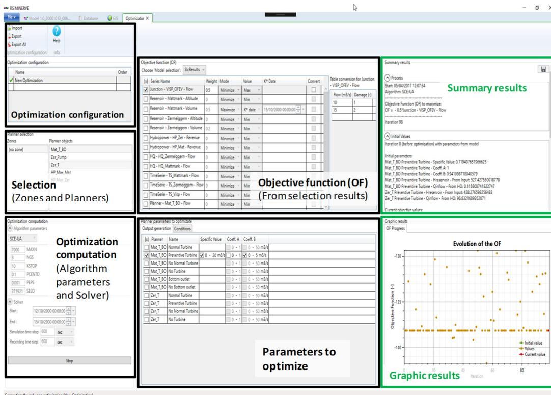
Figure 71 Interface of the Planner optimization module (in black: configuration; in green: results)
